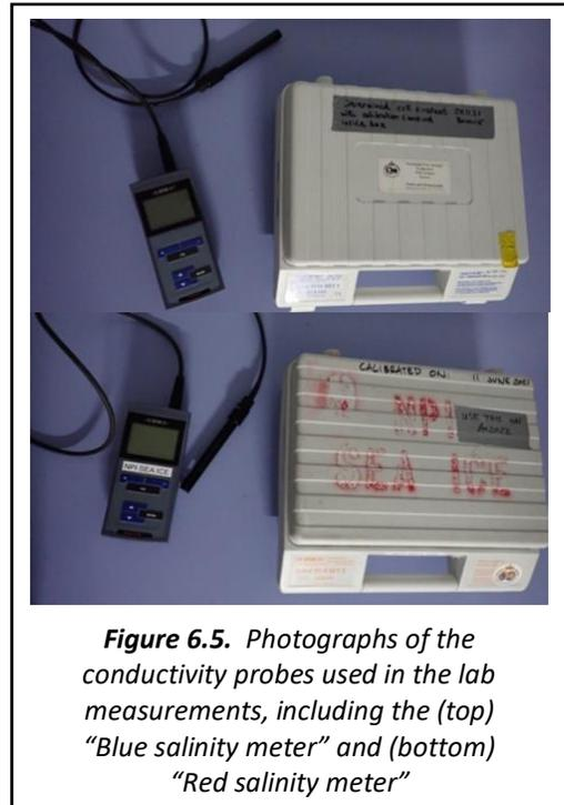
**Figure 6.5.** Photographs of the conductivity probes used in the lab measurements, including the (top) “Blue salinity meter” and (bottom) “Red salinity meter”
