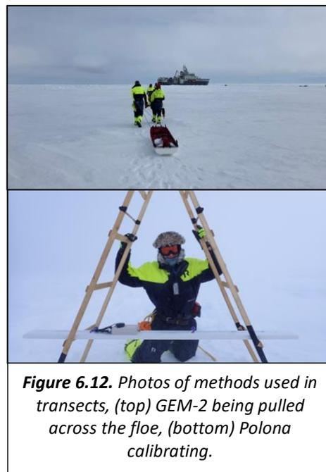
**Figure 6.12.** Photos of methods used in transects, (top) GEM-2 being pulled across the floe, (bottom) Polona calibrating.
