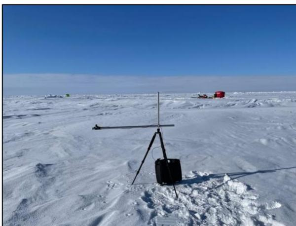
**Figure 6.1** Photo of tripod set-up used to measure albedo and log surface downwelling of PAR
